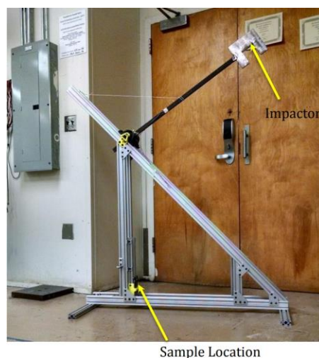
Fig. 2. Charpy impact tester schematic
