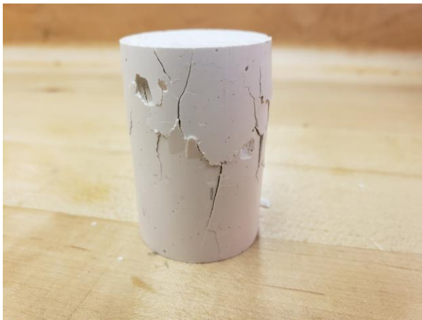
Fig. 2: Plaster of Paris sample after failure. Vertical cracks can be observed running through the sample. Sample also presents brittle characteristics.
