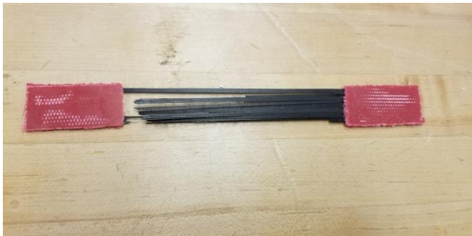
Fig. 6: Carbon fiber sample after failure. Sample failed in vertical lines along the borders of separate fibers. Single fibers can be seen after failure.
