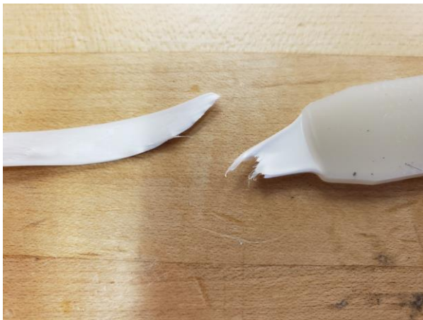
Fig. 8: Nylon sample after failure. The sample was stretched significantly more than all the other materials, necking can be observed.
