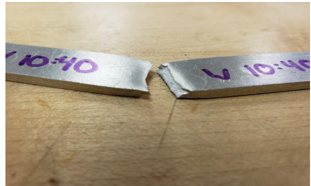
Fig. 4: Unknown metal sample after failure. The sample failed in a plane angled at 45°
